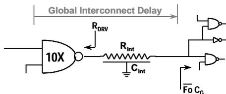
Figure 8. Circuit diagram of a synthetic global net
