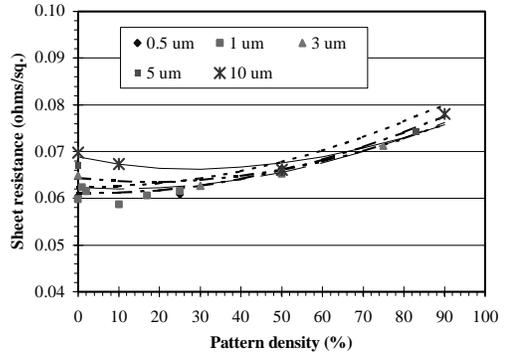
Figure 5. Impact of pattern density on metal resistance (symbols are experimental data and lines show the empirical model)
