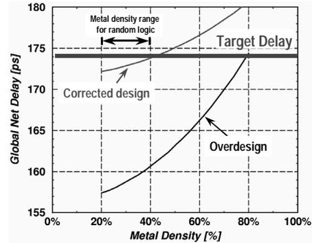
Figure 9. Variation of the synthetic global net reference circuit as a function of pattern density
