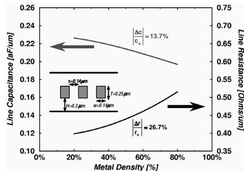
Figure 6. Variation of interconnect capacitance and resistance as a function of pattern density
