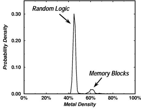
Figure 2. Probability density function of interconnect pattern density of M1 metal layer shown in Figure 1
