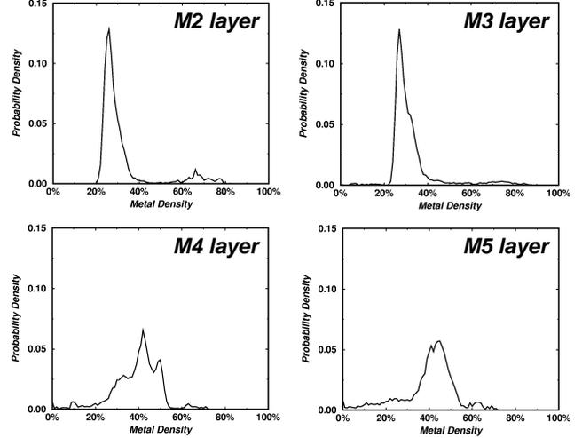
Figure 3. Probability density function of wiring pattern density of M2 to M5 metal layers
