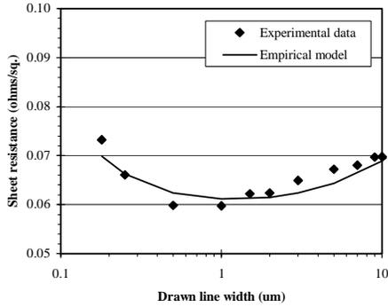
Figure 4. Effect of line width on metal sheet resistance for isolated lines
