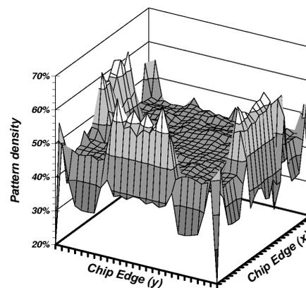
Figure 1. Pattern density of M1 metal layer in a real ASIC chip with 100 $\mu$ m window size
