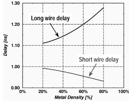
Figure 7. Variation of short and long interconnect delay as a function of pattern density
