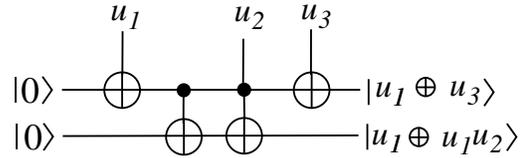
**Figure 5: An example of a ROM-based circuit diagram. The variables at the top of the diagram are the ROM bits.**
