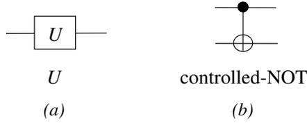
**Figure 1: Circuit diagram for (a) an arbitrary one qubit gate, and (b) a controlled-NOT gate.**
