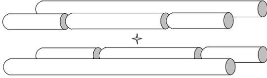
**Figure 2: Schematic diagram of a linear Paul trap, consisting of four parallel rods. A radio-frequency voltage is applied to the continuous rods, while the segmented rods are held at a DC potential. The star indicates the position of the ion(s).**
