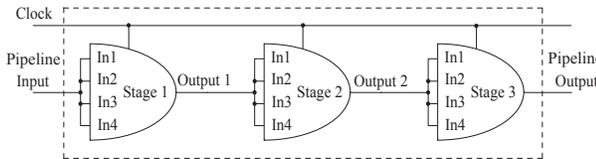
**Fig. 3. Three stage pipeline of four input domino AND gates.**
