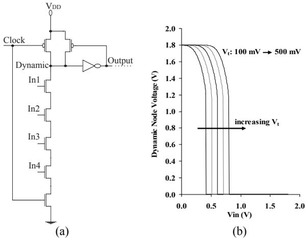
**Fig. 1. Domino logic circuit and voltage transfer characteristics (VTC). (a) Standard domino logic circuit with a keeper (SDK). (b) VTC of SDK for various threshold voltages.**
