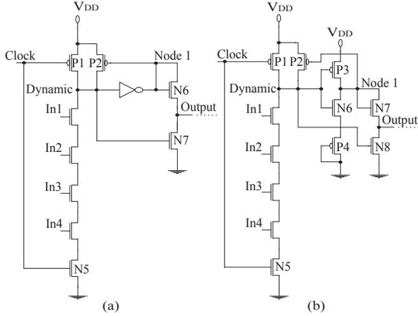
**Fig. 2. The proposed low swing domino logic circuits. (a) Low Swing Domino Circuit with Fully Driven Keeper (LSDFDK). (b) Low Swing Domino Circuit with Weakly Driven Keeper (LSDWDK).**
