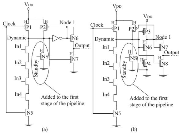
**Fig. 5. Dual threshold voltage implementation of the proposed low swing domino circuits. (a) Dual- $V_t$  LSDFDK. (b) Dual- $V_t$  LSDWDK.**
