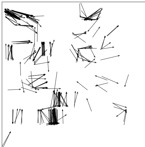
Figure 3: Displacements made by GLS on the PU circuit after 12 hours. At the top are shown the displacements from 0% to 2% of the maximum displacement. In the middle the displacements from 2% to 6% and at the bottom the displacements which are longer than 6%.
