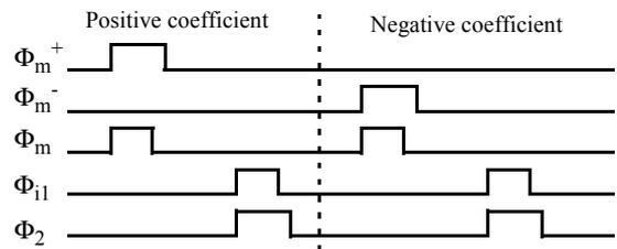
Figure 8: Clock waveforms to perform a MAC operation with positive and negative coefficients.
