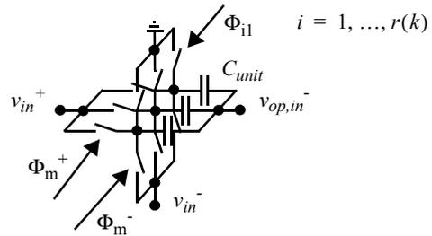
Figure 7: Elements in the programmable capacitor array (PCA), attached to the node  $v_{op, in}^-$ .
