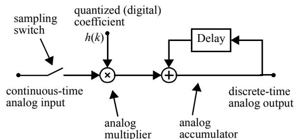
Figure 1: Signal flow graph of the mixed analog/digital MAC unit.
