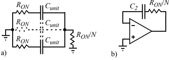
**Figure 10: The simplified SC circuit in its a) multiplication and b) accumulation phase.**
