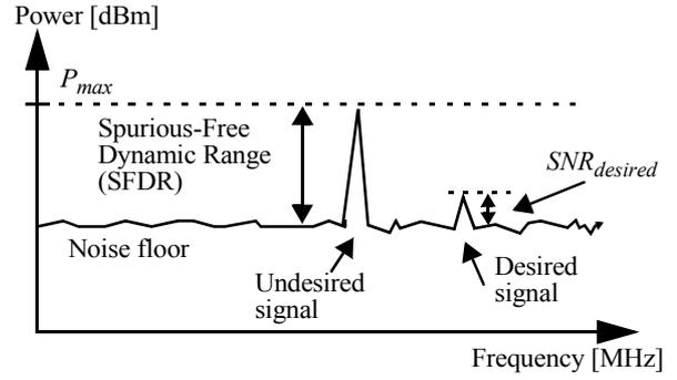
**Figure 5: Typical environment with a weak desired signal and a strong undesired signal.  $P_{max}$  is the maximum power allowed.**
