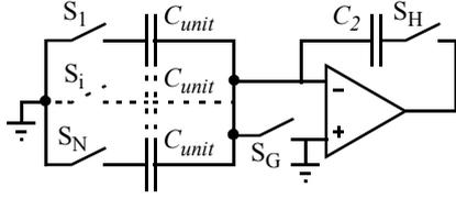
**Figure 9: The single-ended SC circuit used for thermal noise analysis.**
