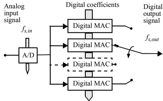
Figure 3: Mixed-signal system I. The traditional realization of a mixed-signal system comprises an A/D converter in the front-end and  $K$  parallel all-digital MAC units.
