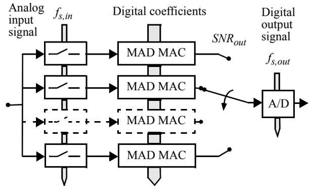
Figure 4: Mixed-signal system II. The proposed realization of a mixed-signal system comprises  $K$  parallel MAD-MAC units, and an A/D converter or a quantizer in the back-end. The MAD-MAC units include track-and-hold circuits.
