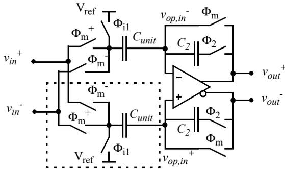
Figure 6: A fully differential MDAC with a PCA consisting a single element.
