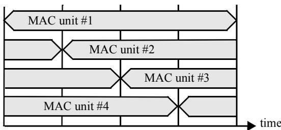
Figure 2: Scheduling of computations on four MAC units. Each output value is a linear combination of sampled input data and digital controllable coefficients.
