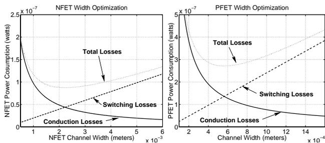
Fig. 9. Switch Optimization Curves
