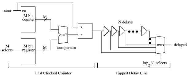
Fig. 10. Controller Block Diagram
