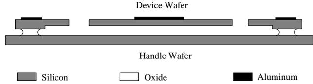
Fig. 4. MEMS Device Side View (Not to Scale)
