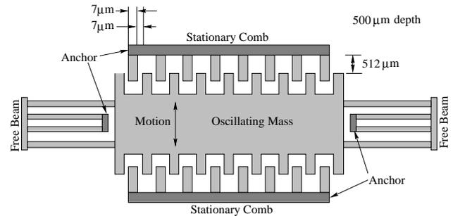
Fig. 5. MEMS Device Plan View (Not to Scale)
