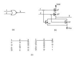
Let  $T=\{\overline{D},0\}$  be a transition cube. Then,  $T(1)=\{0,0\}$ ,  $T(2)=\{1,0\}$ . It is easy to see that < T(1),T(2)> is a robust test for the  $n_1$  stuck-open fault, and T (which
