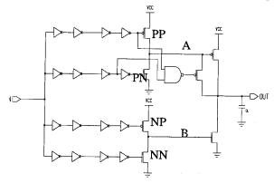
Figure 1. Charge recycling clock buffer circuit
