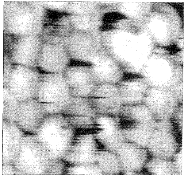
Figure 1. A 43 nm × 43 nm STM topographic image of a close-packed array of 4 nm Au clusters tethered on a GaAs device layer. Image is acquired with a tunneling current of 200 pA and a sample bias voltage of -1.5 V.
