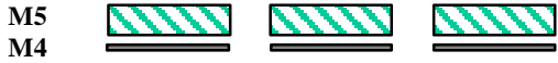
Fig.2 Shows the cross section of the three sub units selected from the body of the inductor in Fig.1. In the meshing of this structure we use 3 vertically stacked layers of sub elements for the thick metal (M5) and 1 layer for the thin metal (M4).
