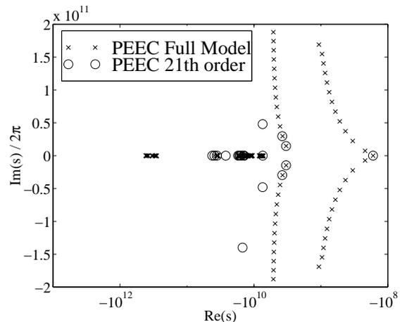
Figure 5: The poles of the transmission line.
