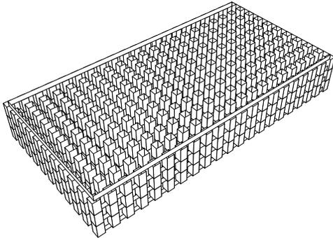
Figure 3: three dimensional discretization of the semiconductor substrate.
