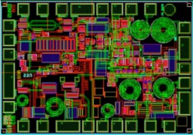
Figure 5: The layout of an RF Front End.
