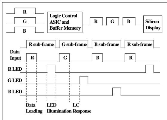
Figure 6. Schematic of the color sequential technique applied to the silicon microdisplay.
