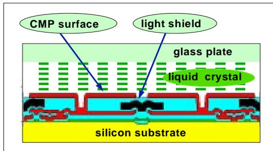
Figure 3. Cross section of the liquid-crystal-on-silicon structure.
