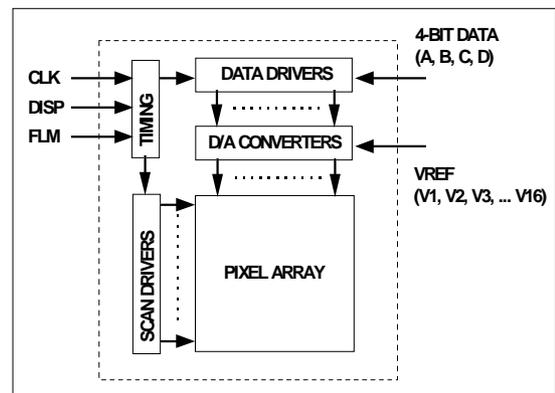
Figure 1. Functional block diagram of the silicon microdisplay panel.
