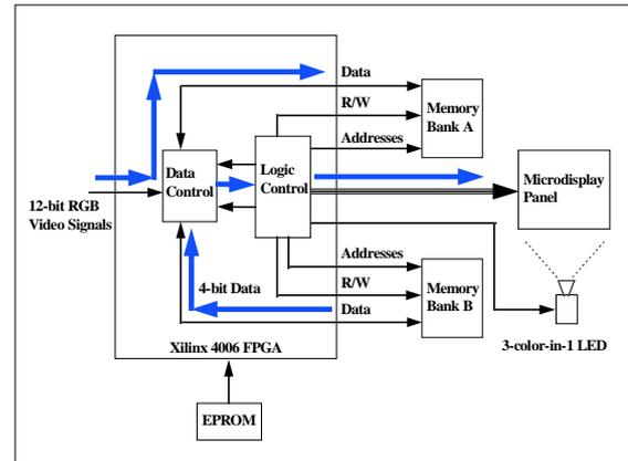
Figure 7. Functional block diagram of the color sequential display system.
