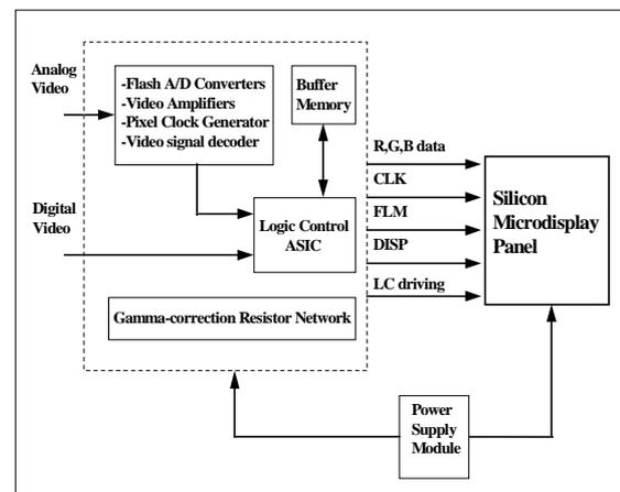
Figure 5. Block diagram of the smart display system.
