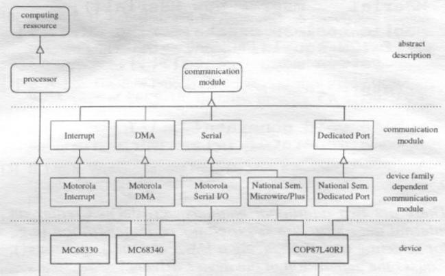
**Figure 5. Object oriented modeling of processors**
