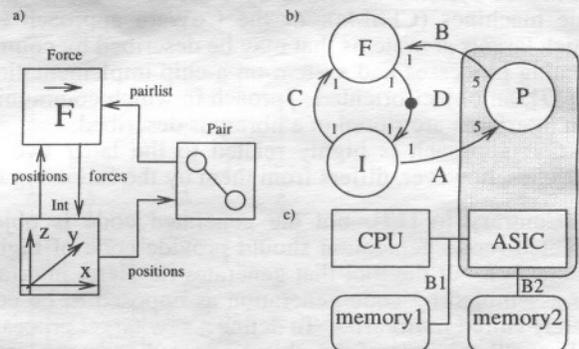
Figure 1. Dataflow graph for molecular dynamics simulation and target architecture
