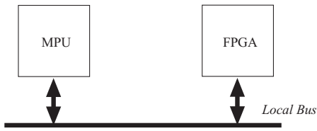
Figure 9. Interconnection using Local Bus VME-BUS
