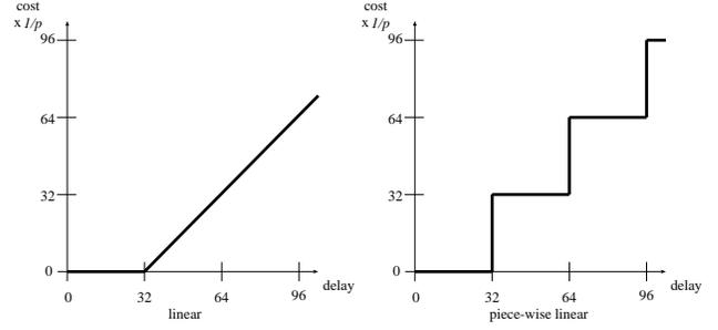
Figure 5: Linear and piece-wise linear cost function for a precedence  $r = (o, o', (p, b, b'))$  with a delay  $d(r)$ .
