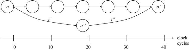
Figure 3: The example from Figure 2 in which the SFG is extended with an extra operation  $o''$  and data precedences  $r'$  and  $r''$  such that the time assignment is feasible.
