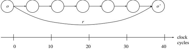
Figure 2: Example of an SFG with a time assignment that is infeasible since the difference between the time of consumption and the time of production of the samples of data precedence  $r$  exceeds the maximum storage time of one silo.
