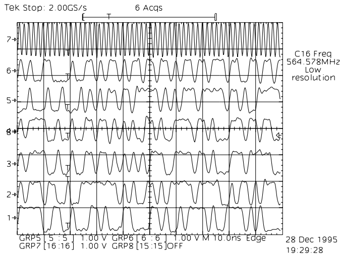
Fig. 7: SOI filter operating at 564 MHz.
