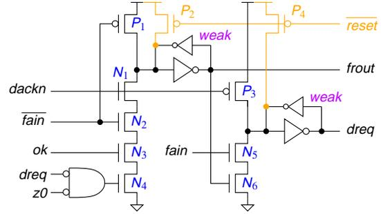
Figure 4: *Biu-fifo2dma* circuit ( $z_0$  and  $z_1$  gates not shown).
