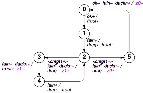
Figure 3: *Biu-fifo2dma* specification with state variable transitions annotated.
