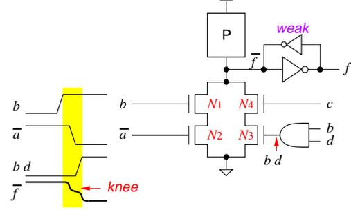
Figure 5: Dynamic hazard in generalized C-elements.
