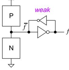
Figure 1: A generalized C-element with a sustainer:  $P \neq \overline{N}$
