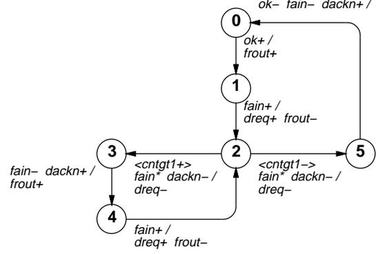
Figure 2: *Biu-fifo2dma* specification.
