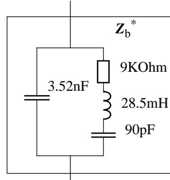
Fig.5 The rough circuit model of piezoelement
