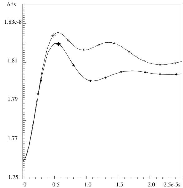
Fig.6 Charge responses of the ANSYS model (◊) and the rough circuit model (+) of piezoelement U1
