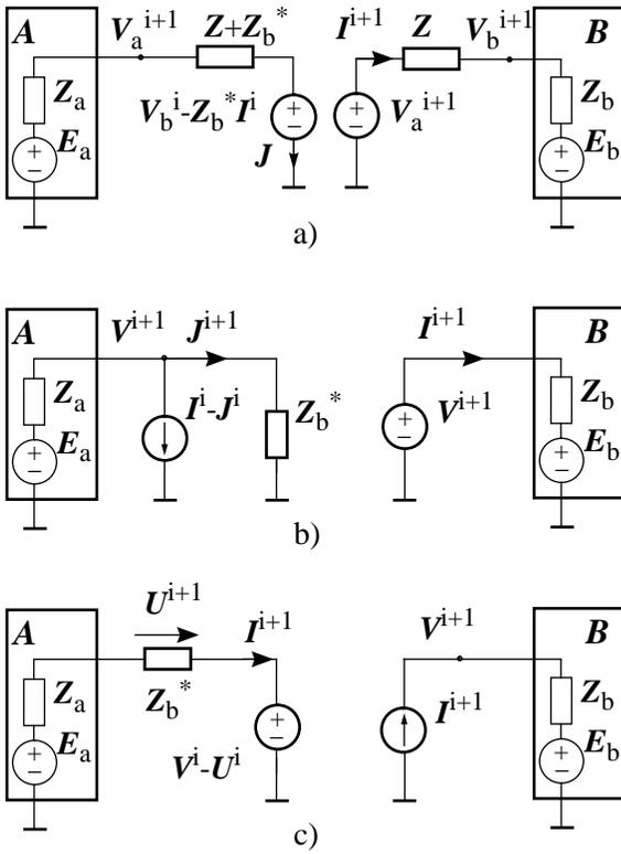
Fig.3 Modified types of coupling in the decomposed circuit
