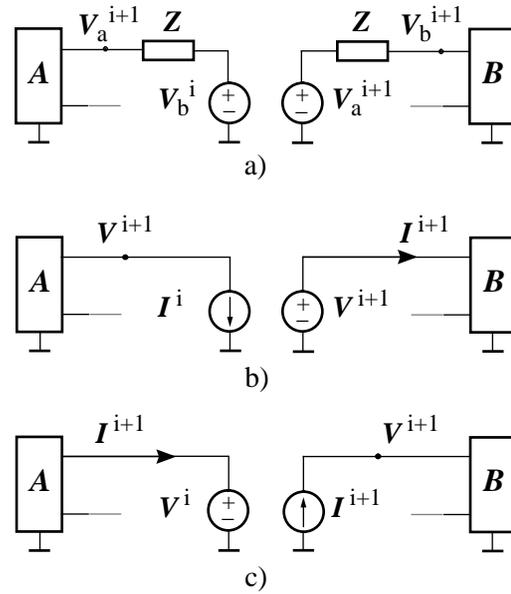
Fig.2 Basic types of coupling in the decomposed circuit
