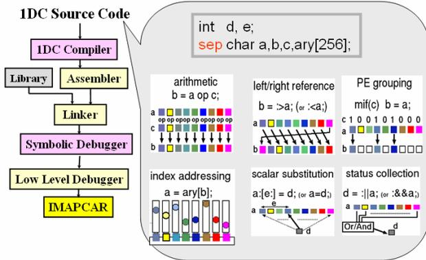
Fig. 6. Six primitive IDC syntax forms (extension from C) and the IDC compiler system
