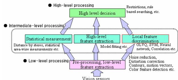
Fig. 3. Processing structure of vision applications.
