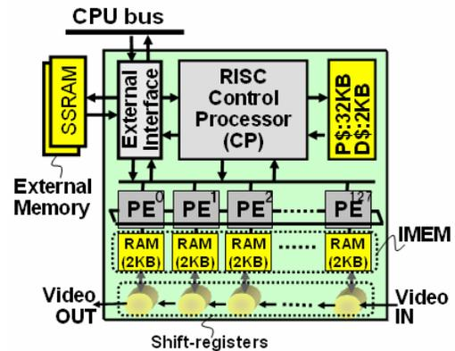
Fig. 4. IMAPCAR block diagram.
