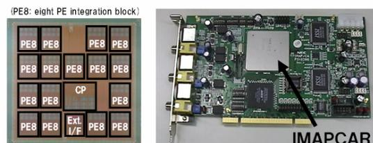
Fig. 5. Die photo and IMAPCAR PCI test board.
