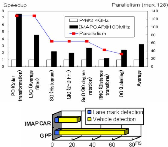
Fig. 8. Speedup ratio of C code running on a 2.4GHz P4 compared with 1DC code running on a 100 MHz IMAPCAR, using various vision tasks.
