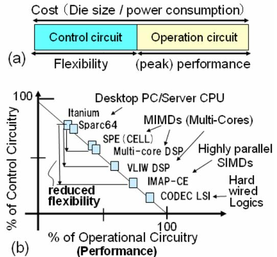
Fig. 1. Relationship between performance, cost, and flexibility, and the Control versus Operational circuit Ratio (COR).
