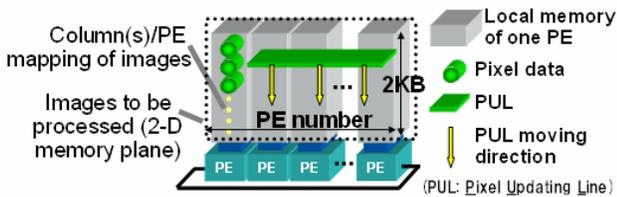
Fig. 7. IMAPCAR program working model
