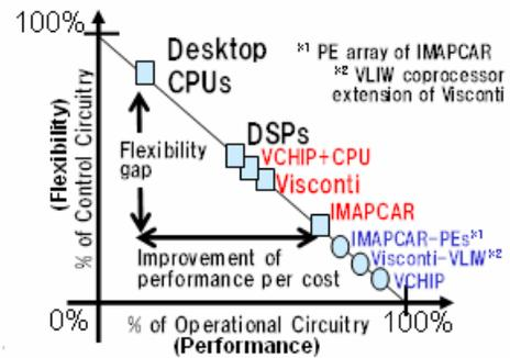
Fig. 9. COR relationship between existing in-vehicle vision processor architectural design approaches.
