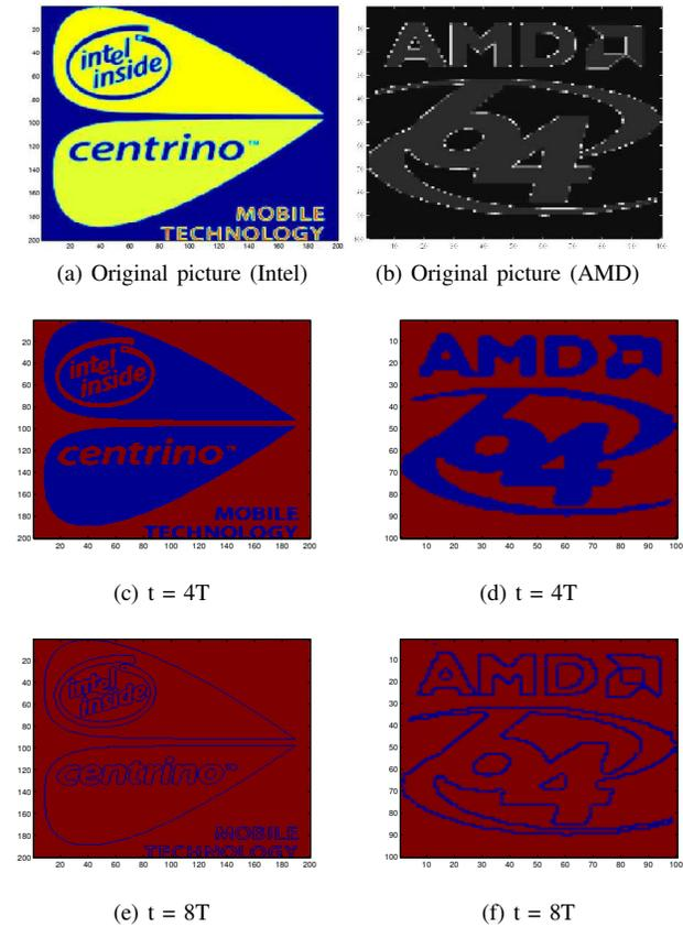
Fig. 10. Image edge detection performed by a TPL-CNN.
