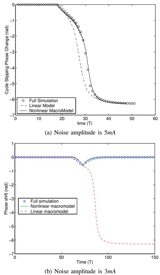
Fig. 5. Cycle slipping in the PLL under different noise amplitudes.
