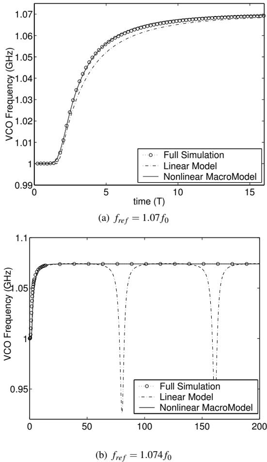
Fig. 4. The step response of the PLL under different reference frequencies.
