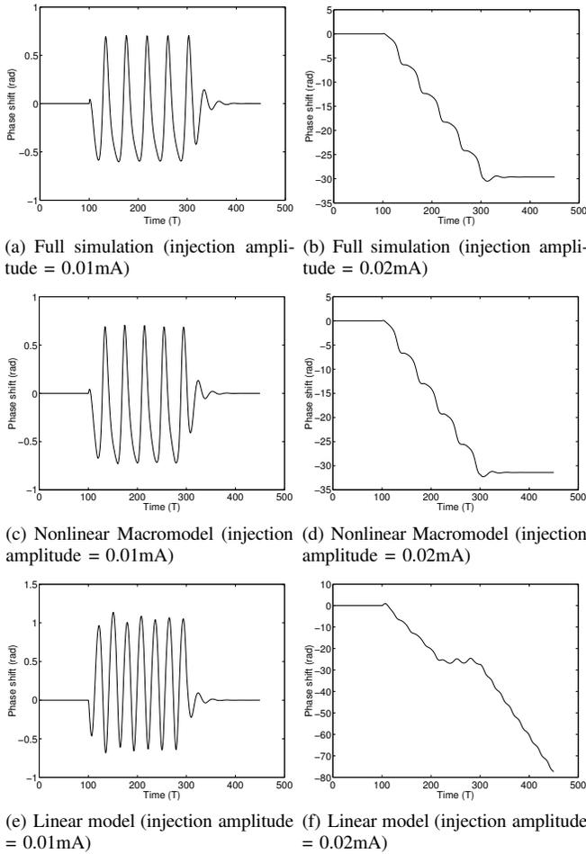
Fig. 6. Phase shift of the PLL under different injection amplitudes, using different simulation methods.
