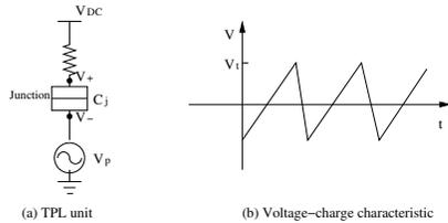
Fig. 9. TPL unit and its voltage-charge characteristic.
