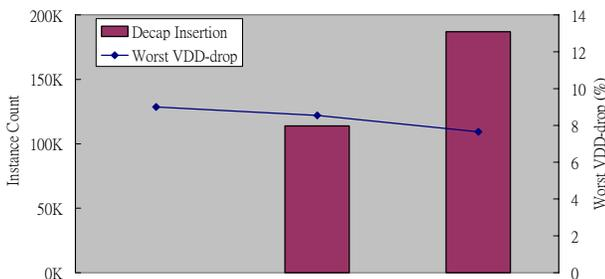
Fig-4 Dynamic IR drop improvement by decap insertion
