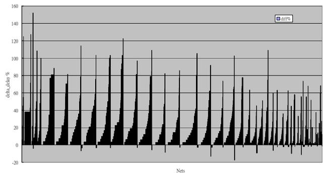
Fig-3 SI timing impact due to dummy metal fills
