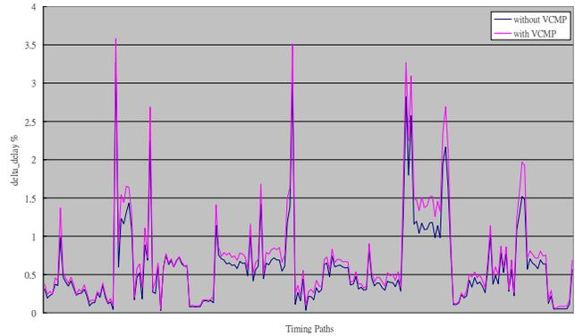
Fig-2 Timing impact due to dummy metal fills
