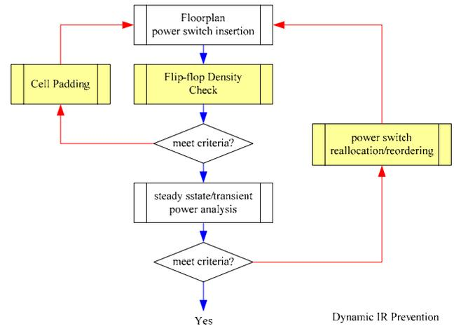
Fig-5 Dynamic-IR prevention during prototyping
