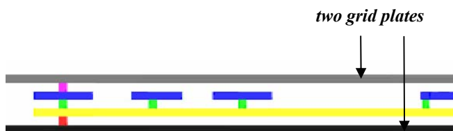
Figure 7. A partial cross-sectional view of the light-colored realnet in Figure 6, which is between two grid plates.
