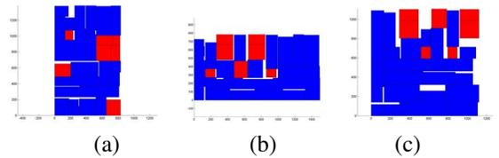
Fig.5 (a) Without constraint; (b) With symmetry; (c) With both symmetry and thermal constraints
