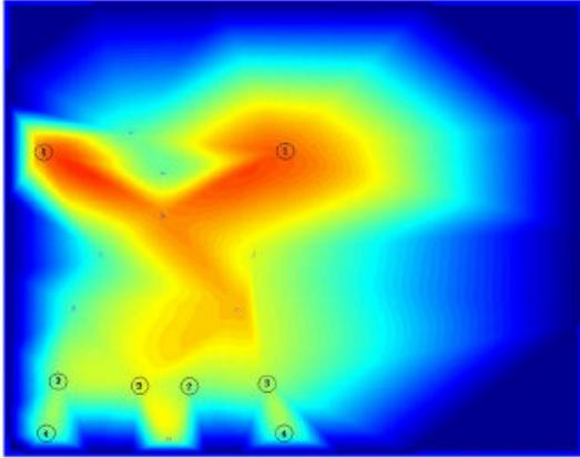
Fig.12 (b) Heat distribution planform with both symmetry and thermal constraints
