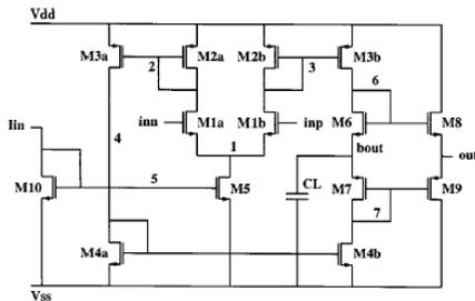
Fig.9 Schematic of a high-speed CMOS comparator
