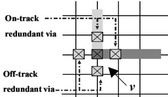
Fig. 8. Illustration of on- and off-track redundant vias.
