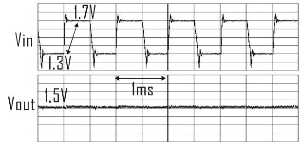
Fig.5 Line transient response of DOC control converter
