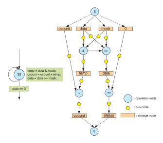
Figure 16. CDFG for state S2 in one's counter
