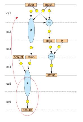
Figure 18. Scheduling process for one's counter (II)
