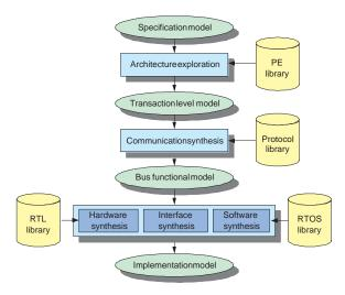
Figure 1. System design flow
