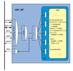
Figure 3. Bus functional model for custom hardware
