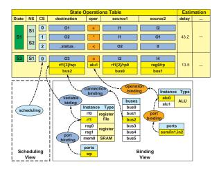
Figure 5. Scheduling & Binding window for an SF-SMD
