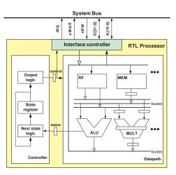
Figure 6. RTL processor architecture
