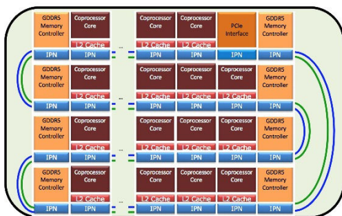
Fig. 1. Intel® Xeon Phi™ coprocessor architecture [1].
