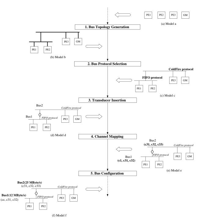
Figure 4. Channel mapping design flow
