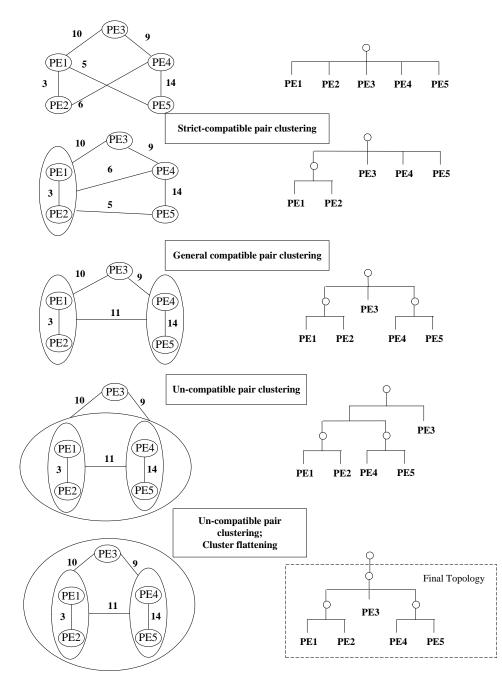
Figure 7. The example of bus topology generation
