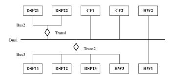
Figure 15. The generated interconnection topology for 10-PE example.
