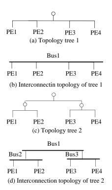
Figure 5. The example of topology tree and interconnection topology
