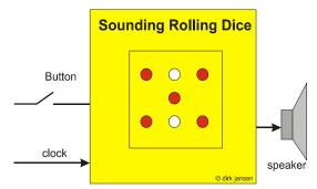
Figure 2: Block-diagram of the sounding, rolling dice.
