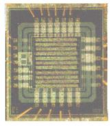
*Figure 20: Standard-cell ASIC of the "Sounding Dice", taken from the authors laboratory [FHO]*
