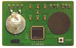
Figure 21: Chip-card size printed circuit board with the "Sounding Dice"-ASIC (in the middle), a speaker (right) and a battery (left), taken from the authors laboratory [FHO].
