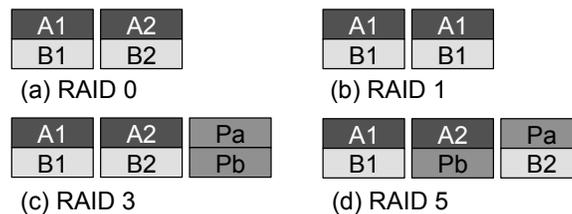
Fig. 3. Sample RAID Levels.
