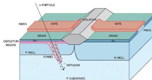
Fig. 1. Soft Error Event Occurrence in CMOS a Device [Lee et al. 2006].
