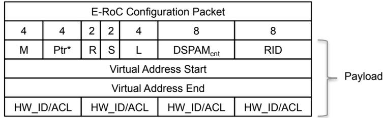
Fig. 13. E-RoC Manager Configuration Packet.
