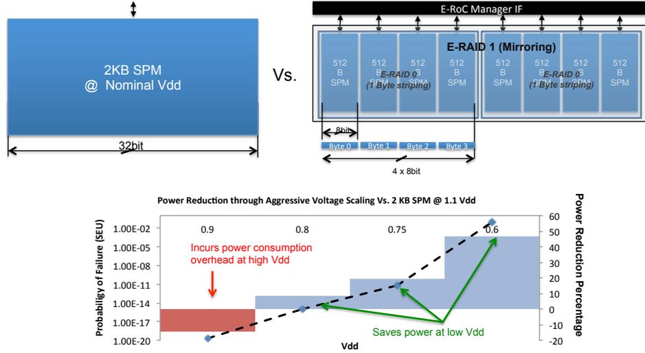
Fig. 6. Power Reduction for E-RAID 0+1 Level.
