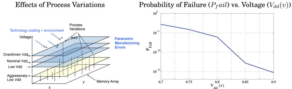
Fig. 2. Effects of Voltage Scaling [Kurdahi et al. 2010] (right) and Probability of Failure due to Voltage Scaling [Sasan et al. 2009a] (left).
