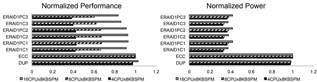
Fig. 17. Normalized performance (left) and power consumption (right) for a pipelined JPEG Encoder using different platform configurations with E-RoC manager support as shown in Figure 9 .
