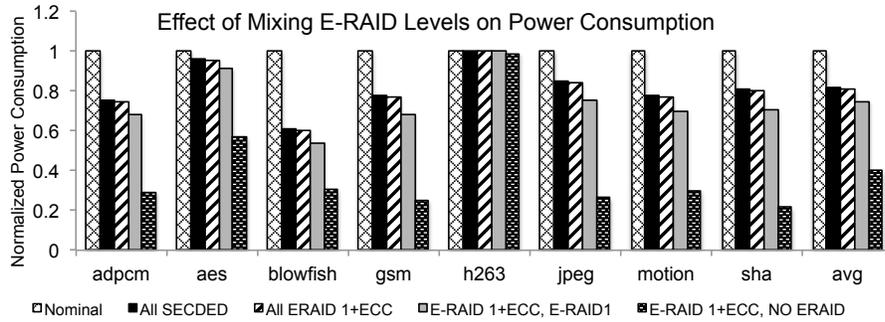
Fig. 28. Effects of Mixing E-RAID's on Power Consumption.
