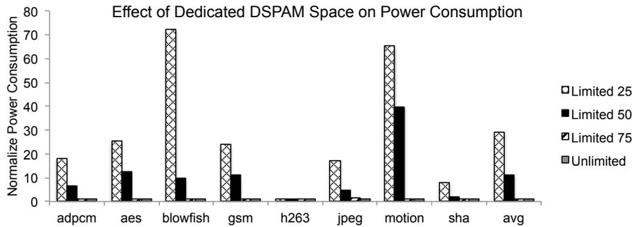
Fig. 26. Effects of Limited DSPAM Space on Power Consumption.
