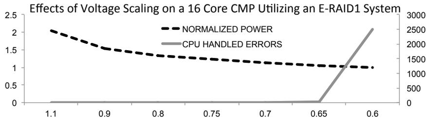
Fig. 18. Effects of Voltage Scaling on E-RoC.
