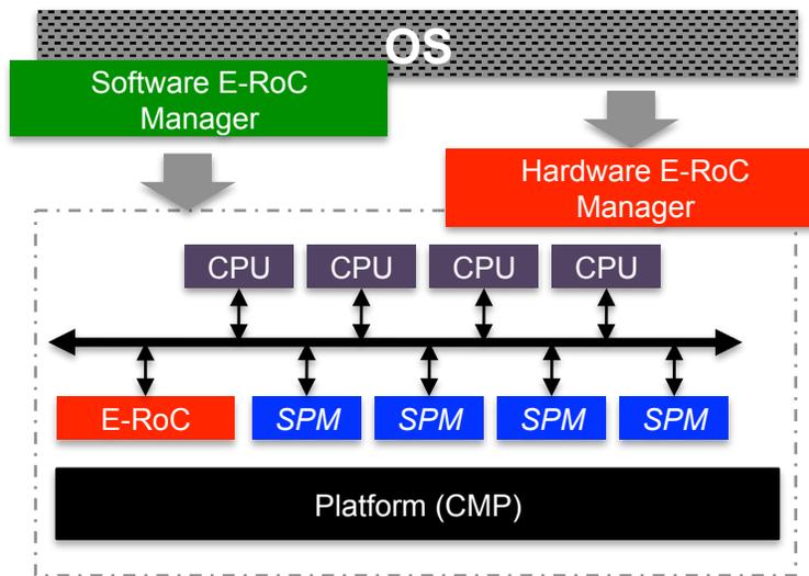
Fig. 15. Software/Hardware E-RoC Layer.
