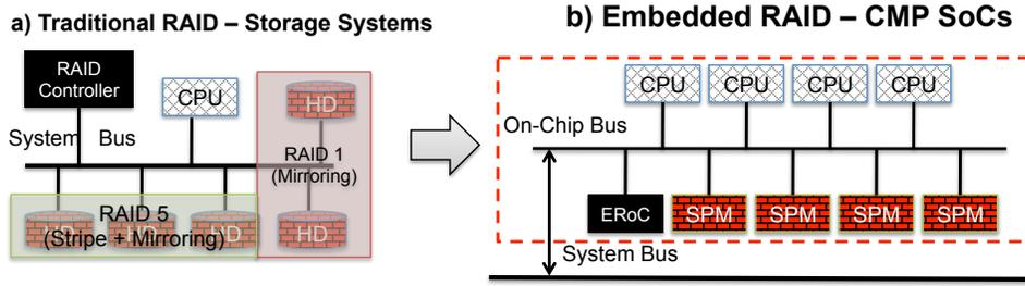
Fig. 4. Traditional RAID vs. Proposed Embedded RAIDs-on-Chip.
