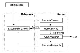
Figure 3: Phases of the SpecC Kernel
