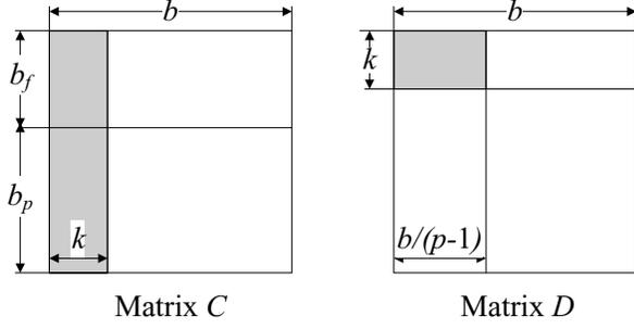
**Figure 3. Workload partition for multiplying one column stripe of  $C$  and one row stripe of  $D$**
