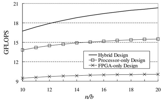
**Figure 8. GFLOPS of LU decomposition vs.  $\frac{n}{b}$  ( $b = 3000$ )**
