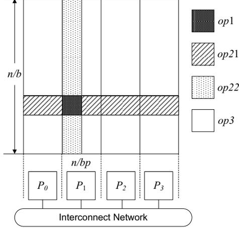
**Figure 4. Illustration of operations of the nodes for Floyd-Warshall algorithm ( $\frac{n}{b} = 8$ ,  $p = 4$ ,  $t = 2$ ).**
