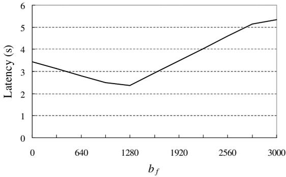
**Figure 5. Latency of one  $b \times b$  block matrix multiplication vs.  $b_f$  ( $b = 3000, p = 6$ )**
