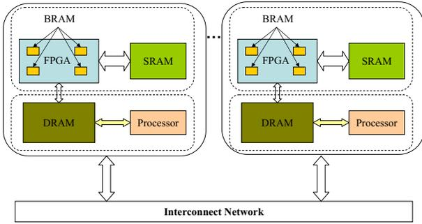
**Figure 1. Architectural Model for Reconfigurable Computing Systems**
