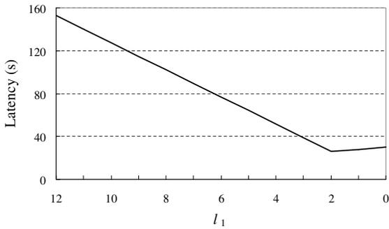
**Figure 7. Latency of one iteration in Floyd-Warshall algorithm using our design vs.  $l_1$  ( $b = 256, n = 18432, p = 6$ )**
