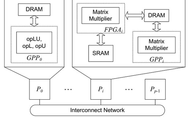
Figure 2. Architecture of our design for LU decomposition in 0th iteration
