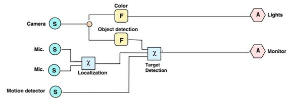
**Fig. 1.** A media processing workflow: “S” denotes sensors, “F” filters, “ $\chi$ ” fusion operators, and “A” actuators
