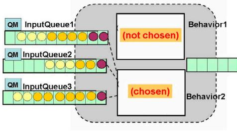
**Fig. 2.** An operator with three input queues and two behaviors; only one behavior will operate on the selected (darker shaded) input objects. Each queue is overseen by a queue manager, which may shed some of the objects (light shaded)
