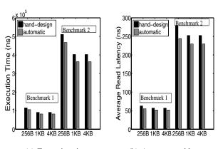
(a) Execution time (b) Average read latency Figure 7: Run time and latency for different cache sizes
