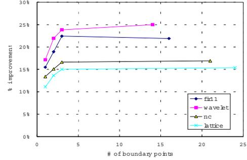
Fig. 6. Effect of multiple boundary points on power improvement.
