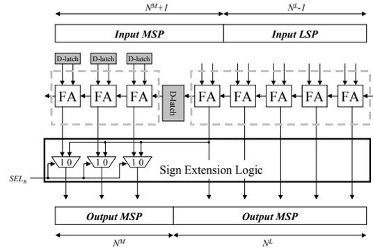
Fig. 3. Partially guarded circuitry for ripple carry adder.
