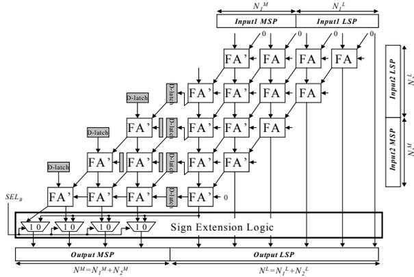
Fig. 4. Partially guarded circuitry for signed array multiplier.
