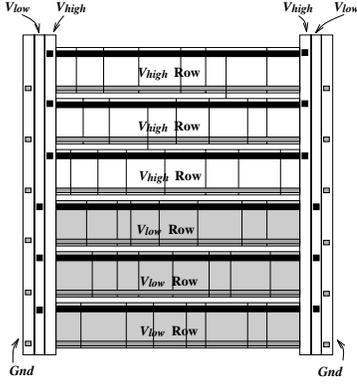
Figure 1: Macro Block Layout Schemes for Voltage Separation
