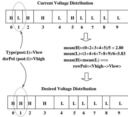
Figure 5: Polarity Computation
