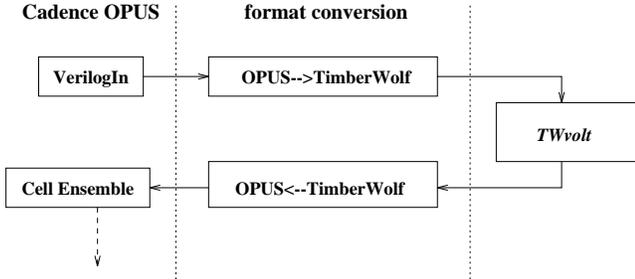
Figure 6: The Layout Design Flow
