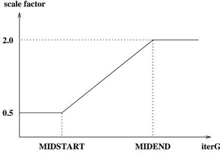
Figure 4: Scaling baseCost to get voltCost
