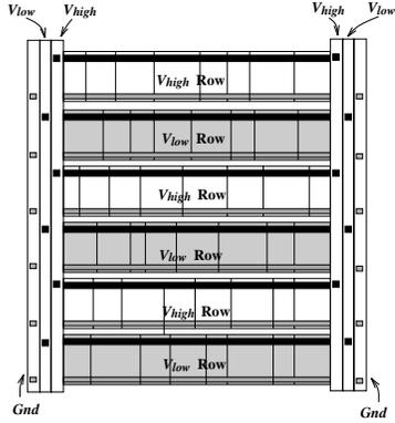
Figure 2: Interleaved Layout Scheme for Voltage Separation
