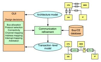
Figure 1: Communication design flow.
