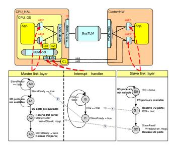
Figure 6: Synchronization by interrupts.
