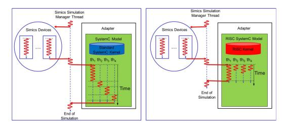
Figure 14: Two different Simics simulations of the same model with the left-side using a standard SystemC kernel and the right-side featuring RISC kernel for out-of-order parallel multithreading of SystemC threads
