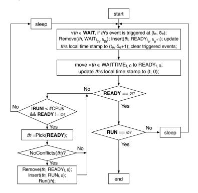
Figure 3: Out-of-Order Parallel Discrete Event Simulation (OoO PDES) scheduler for SystemC.
