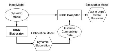
Figure 8: RISC Elaborator feeds dynamic elaboration information to RISC Compiler for precise conflict analysis.
