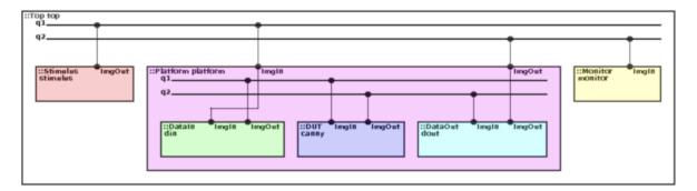
Figure 12: Module hierarchy visualization of a SystemC model of a Canny edge detector.
