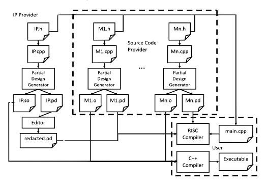
Figure 7: Scaled RISC tool flow with Partial Segment Graph technology.
