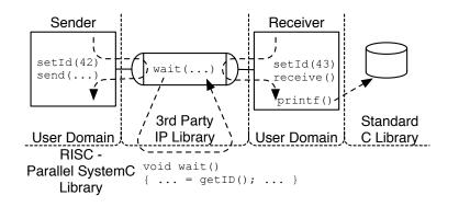
Figure 10: Different source code domains of a design model.
