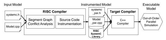
Figure 4: RISC Compiler and Simulator for Out-of-Order PDES of SystemC.
